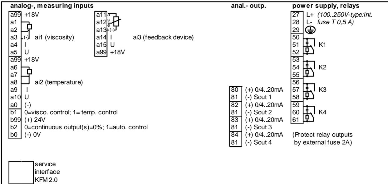
**Wiring, examples for input 1 and output 1 respectively:**
