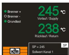
A flashing frame with the description SP shows the activated setpoint level and the parameter name "SP=" the adjusted value as well as a description text optionally.
